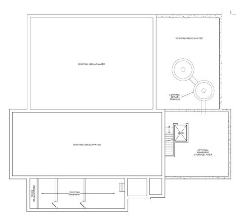
Partial basement under north west addition (bottom right) to include storage area with elevator and stair access.
