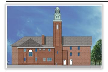
Rear (right side in rendering) to be extended outward with gable roof similar to existing.
